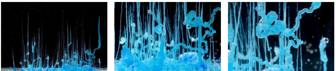
Figure 9: Various stages of the filiform growth of thin copper sulphate crystals which show particularly well the influence of gas bubbles. Wide-angle shot and close-up.
