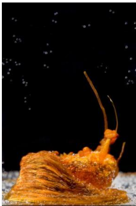
Figure 7: You might think that this is a snail... It is the result of an osmotic growth of iron chloride (III).
