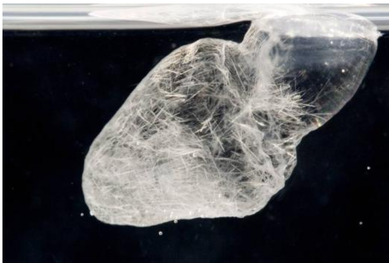
Figure 4: Osmotic cell created by the insertion of a fragment of calcium chloride into a greatly diluted solution. The spikes are microscopic crystallisations, invisible to the naked eye.
