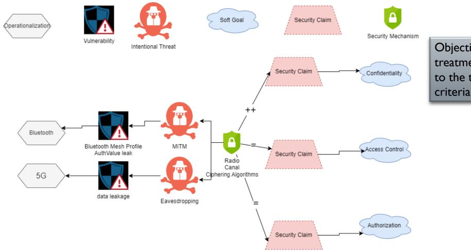
Objective: Link or add the treatments (security mechanisms) to the threats and security criteria
