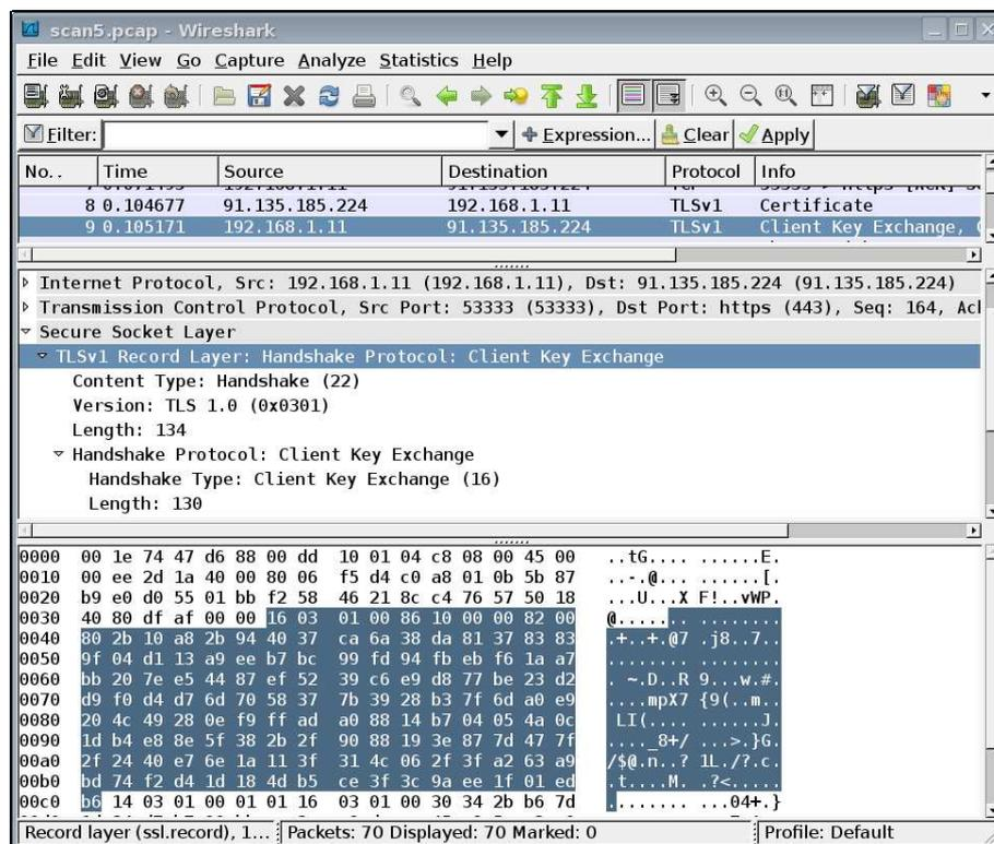
FIGURE 4.25 – Client Key Exchange
